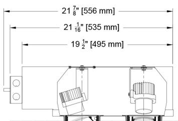
NOTE: This option is intended for use with precise and finished cutouts - usually millwork or wood ceilings. There is no plaster or finish flange.
